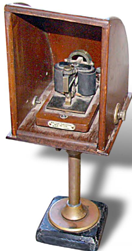
*A sounding relay mounted in a simple wooden box to direct the sound to the operator’s ear; photographed at the Alice Springs Telegraph Station, 2009 [Photo: Richard Venus, 5628]*
