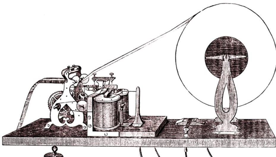
*Samuel Morse's first telegraph receiver: a pen made marks on a paper tape drawn under it by a clockwork mechanism [Prescott, 1866, p423]*
