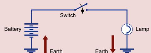
The first circuit is like a recirculating system in an aquarium whereas the "earth return" circuit is like pumping water from a dam. When you open the tap (equivalent to closing the switch), water flows onto your garden. It will keep flowing because water coming from somewhere else keeps the dam full to supply the pump.
